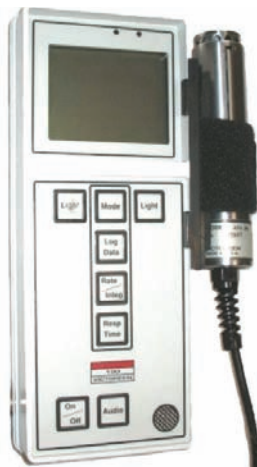
Figure 17: Example of a typical radiation survey meter.
