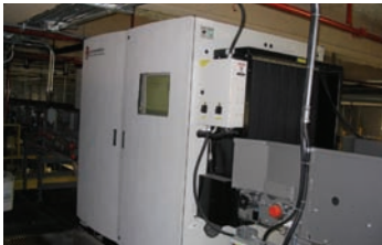
Figure 15: VIS and VDS x-ray machines. The in-line VIS108 machine is shown on the left and the stand alone VDS108 machine used for check-in of oversized baggage is shown on the right.
