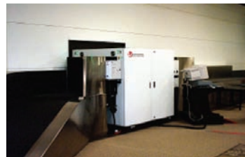
Figure 15: VIS and VDS x-ray machines. The in-line VIS108 machine is shown on the left and the stand alone VDS108 machine used for check-in of oversized baggage is shown on the right.
