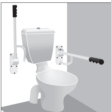
Drop down grab rails on both sides of toilet – generally positioned 200–300mm above toilet seat and 400mm from centreline of pan.
