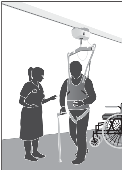
Fixed overhead ceiling hoist for walking a patient in rehabilitation
