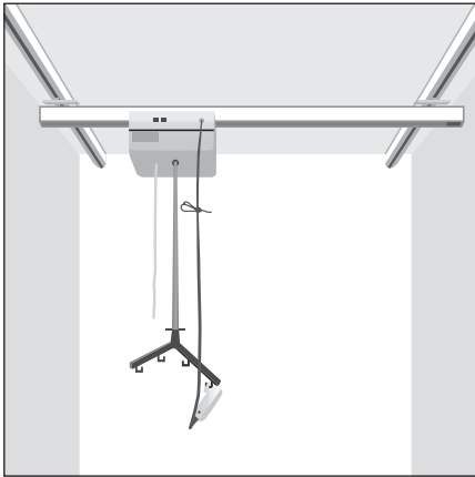
Fixed overhead ceiling tracking and hoist system
