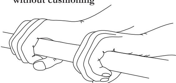
Figure 4.8 Cushioned handles can reduce contact stress and vibration, and increase worker comfort.
