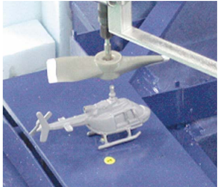
Figure 2: Wind tunnel testing of helicopter model
