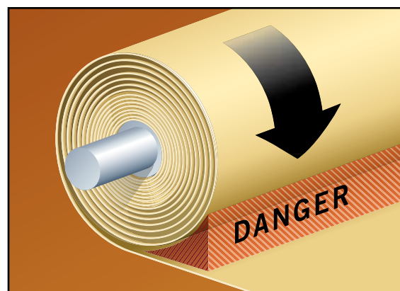
FIGURE 6-4: IN-RUNNING NIP CREATED BY THE WINDING OF MATERIAL
