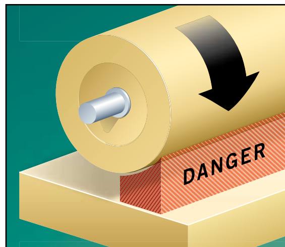
FIGURE 6-3: IN-RUNNING NIP CREATED BY A CYLINDER CLOSE TO A STATIONARY OBJECT
