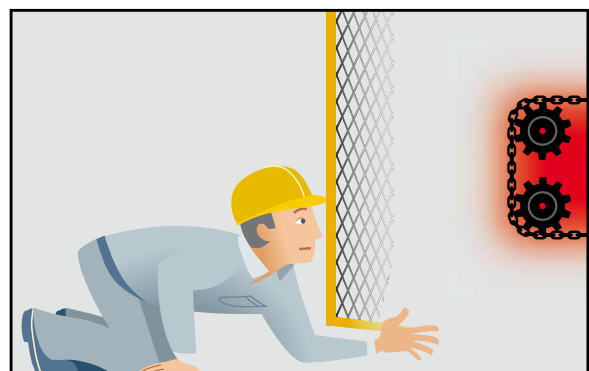
FIGURE 5-11: ACCESS FROM BELOW A GUARD
