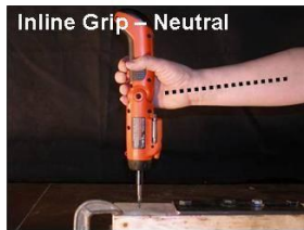
Figure 20. Examples of situations in which a pistol grip and inline grip would be useful as a means for keeping the wrist in a neutral posture.
