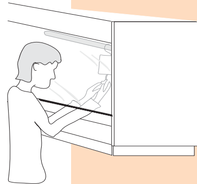
Many biological safety cabinets have a sash window that restricts arm motions.
