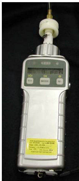
Figure 3.6. ppb-RAE with 25-mm Filter Holder
