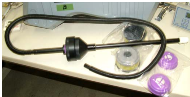
Figure 3.7. Larger Filters Used on MIRAN Analyzers
