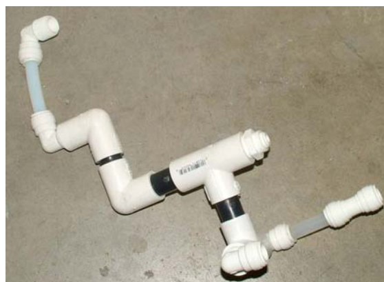
Figure 3.5. Second-Generation Manifold Constructed of PVC and ABS Plastic Fittings and Teflon Tubing
