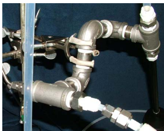
Figure 3.9. Third-Generation Stainless Steel Mixer and Manifold
