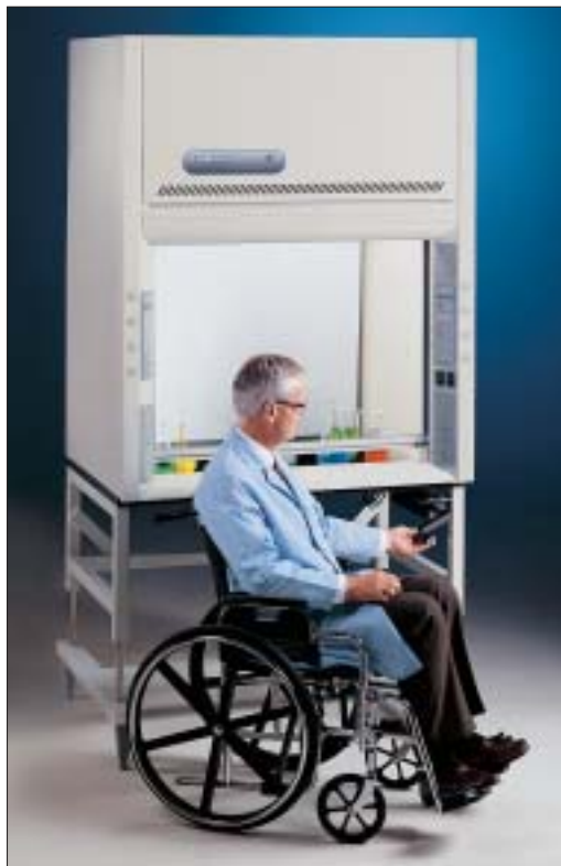
Protector® XL Laboratory Fume Hood on Manual Hydraulic Lift Base Stand may be lowered to accommodate wheelchair-bound users. Hoods on adjustable base stands require special modifications to incorporate flexible ducting, wiring and plumbing
