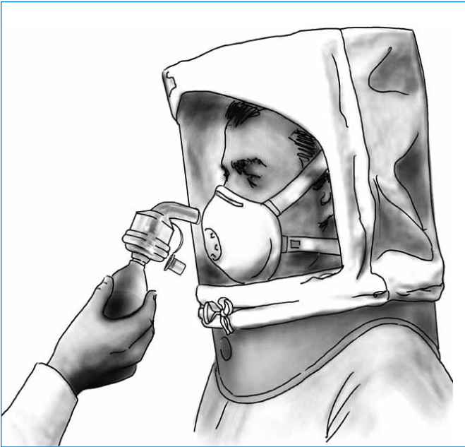
A bitter solution is sprayed into the test hood for the bitter aerosol fit test.
