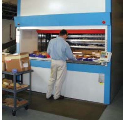
Vertical carousels rotate and present items on shelves or roll out drawers within the worker's power zone.
