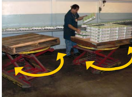
Turntable on a load leveler
